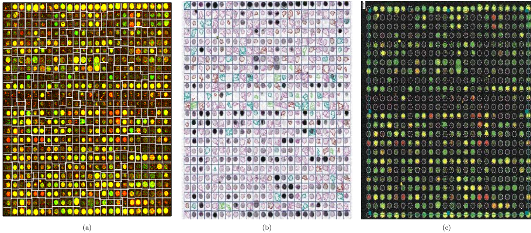
Figure 2: Comparative gridding results of our method (a) with two widely used microarray image analysis tools: (b) the Spotfinder and (c) the ScanAlyze.
