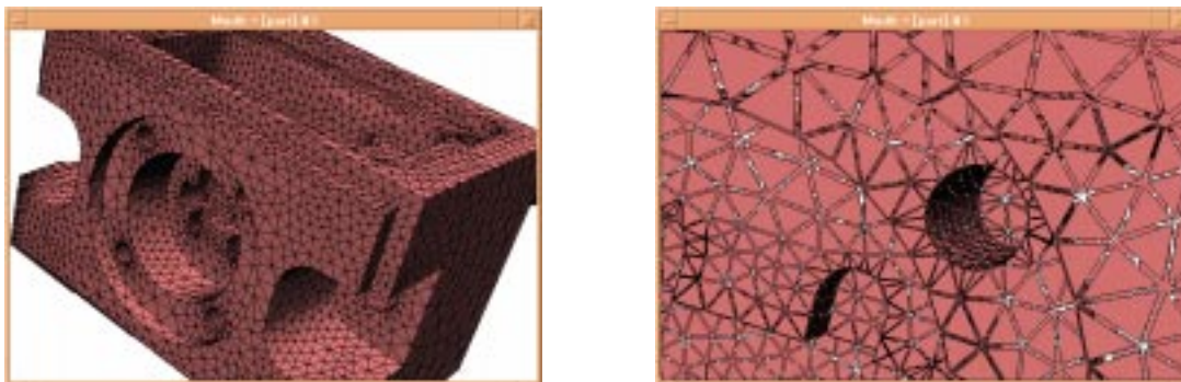
Figure 6: Examples of rendering option : Shading+lines selection (left-hand side) and Shrink flag activated (right-hand side).
