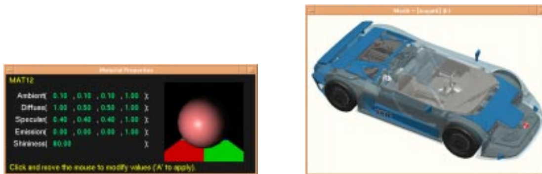
Figure 14: Material edition window (left-hand side) and example of 'realistic' rendering using multiple materials, including transparency effects (right-hand side).
